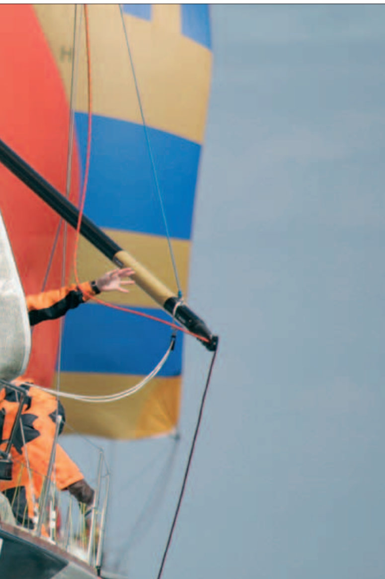
Seldén spinnaker poles are designed to make light work of spinnaker handling. The big advantage of carbon fibre is its low weight. The weight savings enable the crew to handle the spinnaker faster, with less effort.
